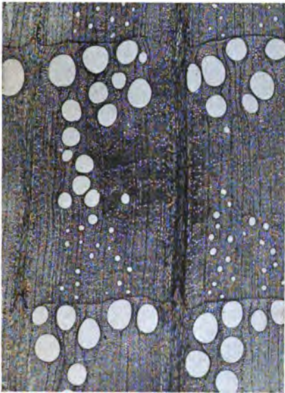
FIG. 329.—Cross-section of Ring-Porous Wood. (Red Oak). (Bull. 126, U. S. For. Ser.)
